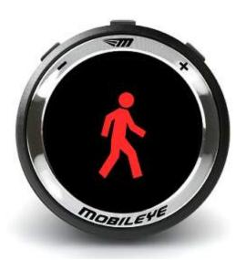
**Pedestrian & Cyclist Collision Warning (PCW) in the Danger Zone** a pedestrian, cyclist or other VRU (Vulnerable Road User) has been detected in the "Danger Zone"; Time-To Collision is not critical.
