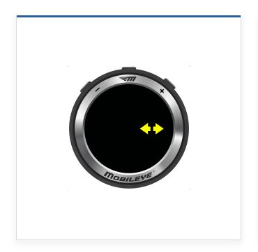
**Turn Signal Reminder** when turn signals are active for a long time, a blinker reminder alert is provided.
