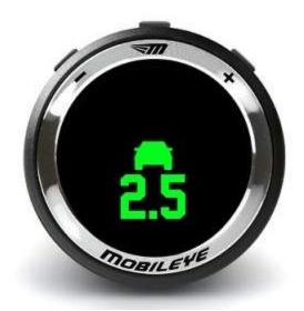
**Pedestrian & Cyclist Collision warning (PCW)** Indicates a possible critical risk of a collision with a pedestrian, cyclist or other VRU (Vulnerable Road User)
