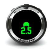
WARNING! A vehicle icon changes to red when the headway is equal to or lower than the predefined headway time threshold, or at 0.6 seconds and lower.
