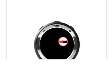
**TSR Minimized Icon** the last detected traffic sign displays as a minimized icon.
