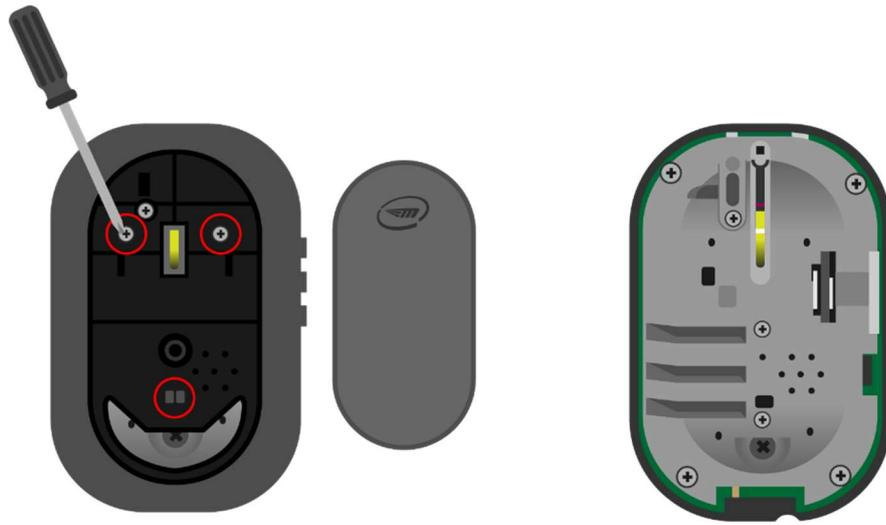
3. Using a Philips screwdriver, unscrew to remove the main chassis from the frame.
