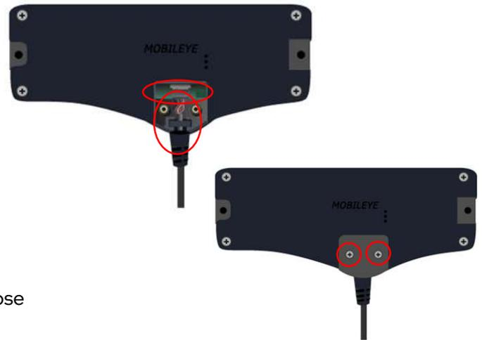
Close the 4G modem connector cover and close the 2 screws
