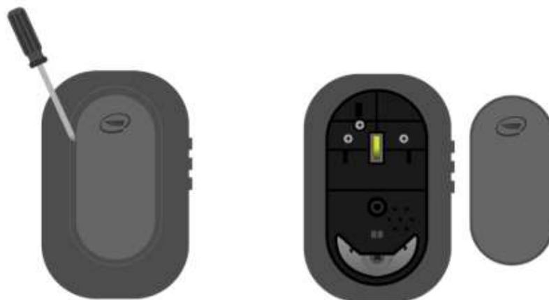
2. Using a Philips screwdriver, unscrew the 3 screws and remove the main back cover.
