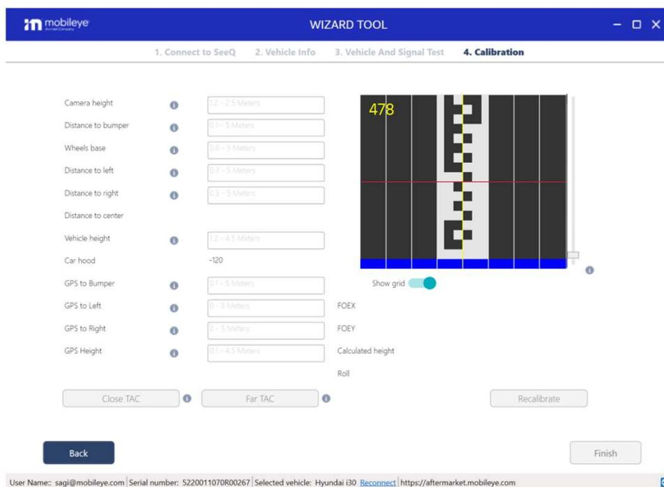
Attach the main camera unit; lining up the IC Wizard **Yellow** line exactly with the camera location on the TAC.
