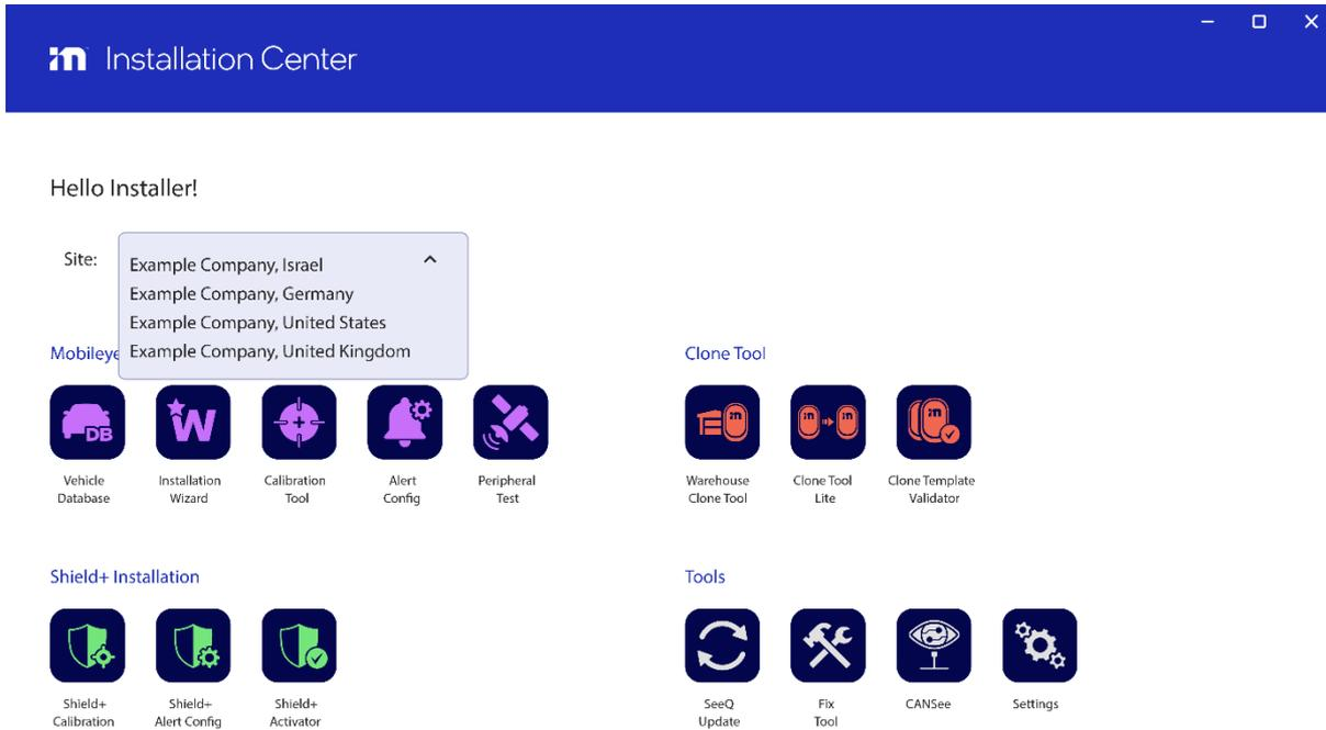
Click the vehicle database icon
