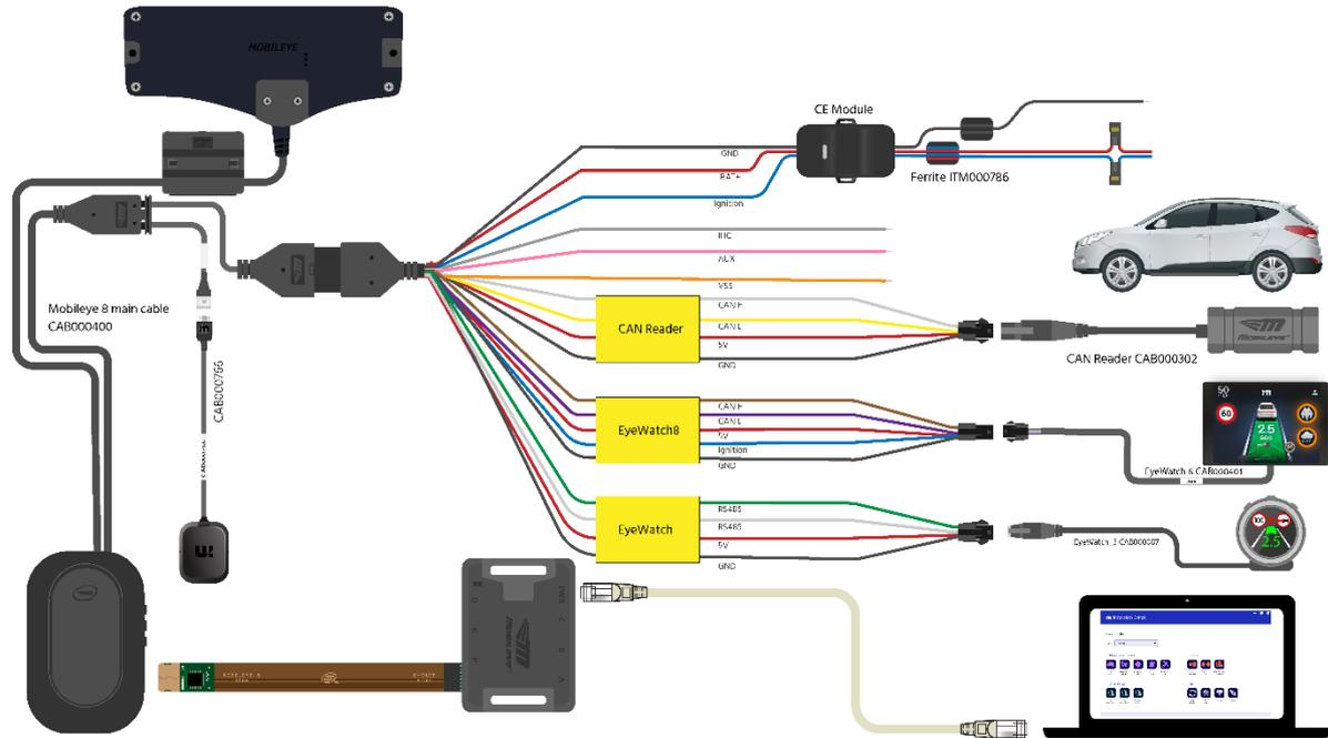
Figure 1 – connection method with EyeNET adapter
