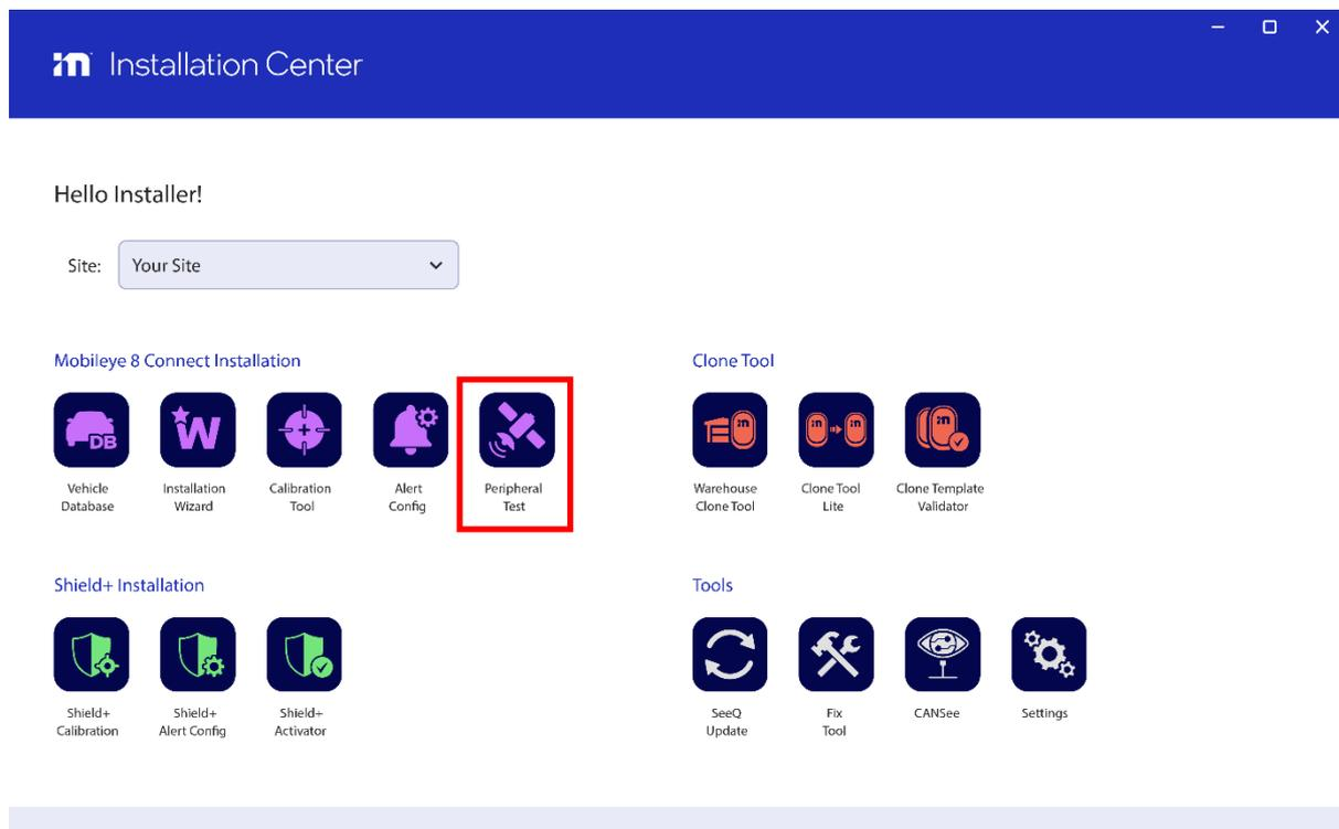
The tool will check communication with the system and display the system s/n and FW version following by the peripherals test and display the status of each component.
