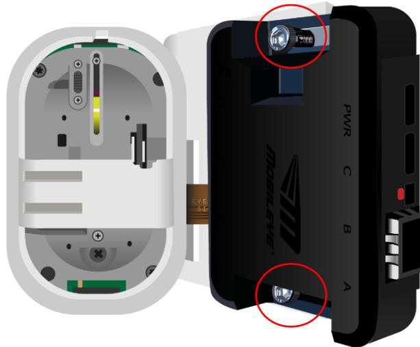
Route the EyeNET flat cable trough the designated gap and connect it in both ends to the Mobileye system and the EyeNET and continue with the calibration process
