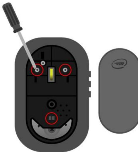
Using a Philips screwdriver, unscrew to remove the main chassis from the frame.
