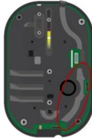
A camera with the new 4G chassis includes silicone cover plug (MEC0001117) to avoid dust and to be used in a case the 4G Modem cable (CAB000405) is routed from the bottom side.
