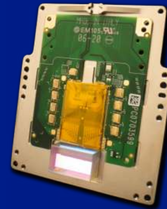
GoldBox- optical head enabling 90 vertical lines per scan
