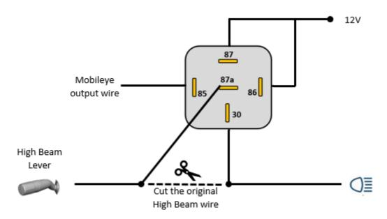
High Beam lever **Negative** polarity
