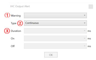
Warning – choose the relevant warning which will be used to trigger the analog output.
