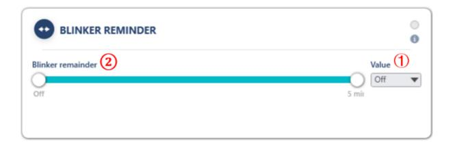
1 By default, BR is set to disable (off). BR activation time can be set to the following values: off, 0.5sec, 1min, 1.5min, 2min, 3min, 4min and 5min.
