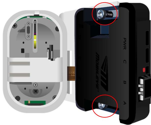
Route the EyeNET flat cable through the designated gap and connect it in both ends to the Mobileye system and the EyeNET and continue with the calibration process
