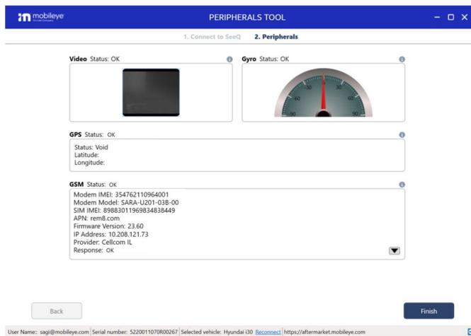
Note that due to the installation location such as underground parking or indoor garage and GPS signal or cellular network is not available, the test status of the relevant component will pass but no valid data will be displayed.
