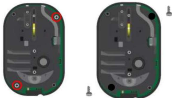
**Warning: Do not unscrew the upper left and lower right screws as it will void warranty!**
