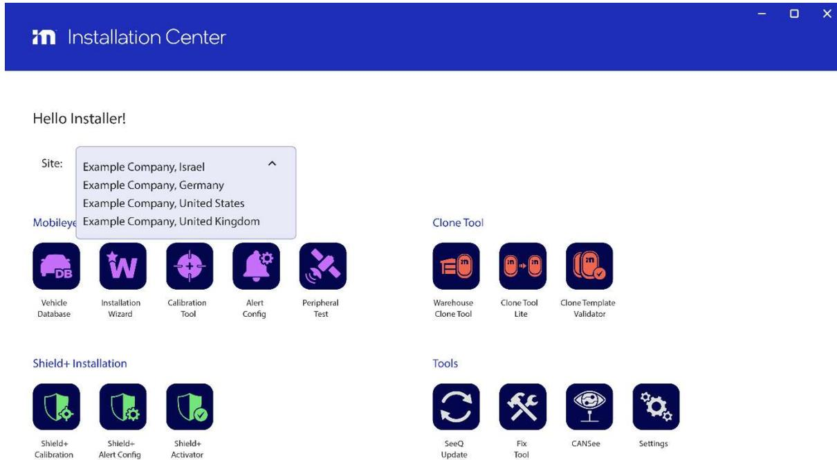
Click the vehicle database icon
