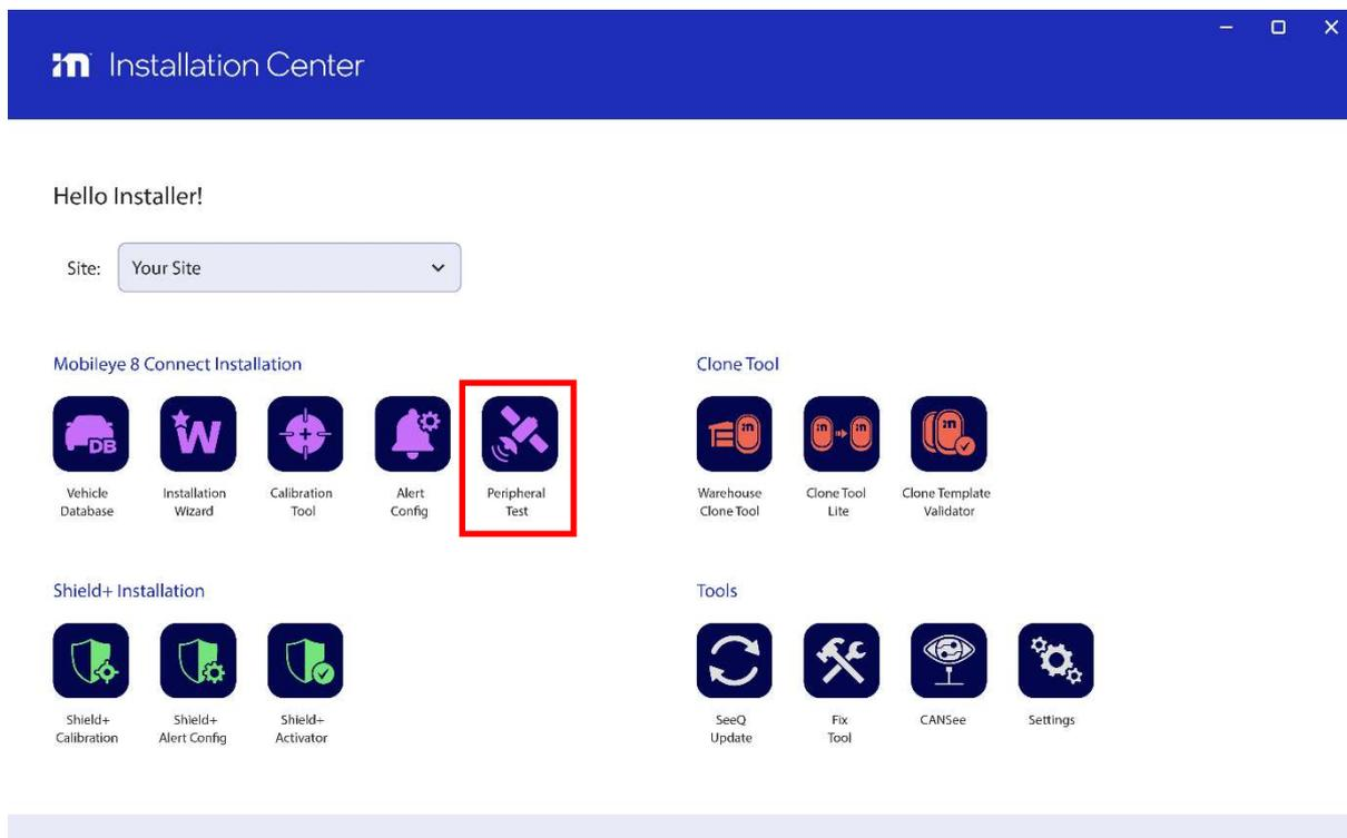
The tool will check communication with the system and display the system s/n and FW version following by the peripherals test and display the status of each component.
