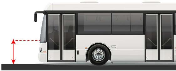
❖ **Distance to bumper** (the distance from the camera to the front bumper).
