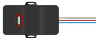
2. Insert each power source from CAB000371 to the dedicated power connection in the CE Module
