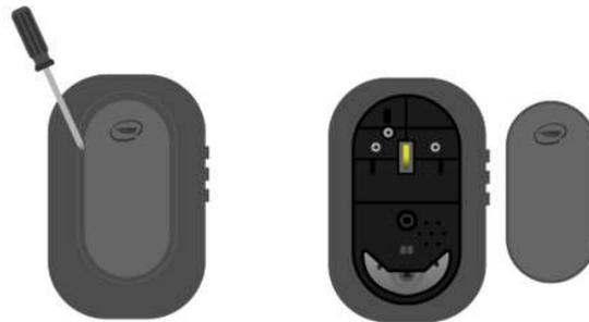
2. Using a small Philips screwdriver, unscrew the 3 screws and remove the main back cover
